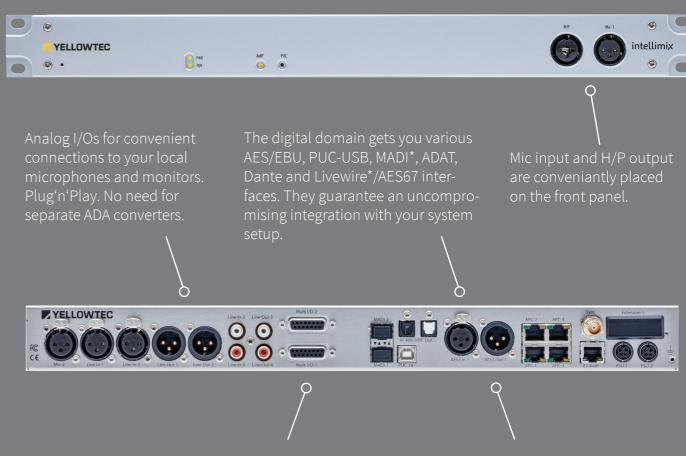
GPI/Os assure flexibility for remote control over various functions. Use them for many convenient logic controls.
