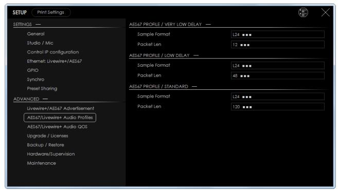
Supported are three profiles with identical settings (but different default values) - Very Low Delay, Low Delay and Standard.
