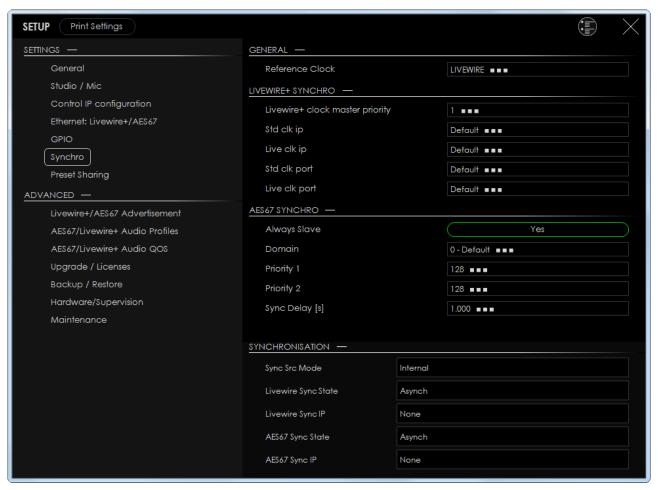
The Reference Clock can be synced either to the LIVEWIRE, Internal or AES67.
