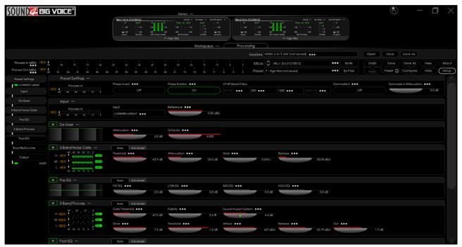
The processing chain also includes: Preset settings, Input, De-Esser, 3-Band Noise Gate, Pre-EQ, 3-Band Processing, Post-EQ, Brick Wall Limiter and Output. The 3-Band Noise Gate and processing sections have an "Advanced" tab that allows access to each band's individual parameters.
