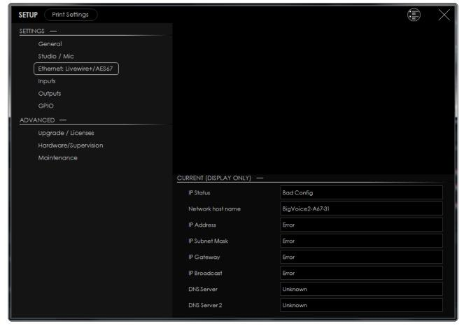
**Current (Display only)** – displays the current information obtained from the device, thus allowing you to verify the applied settings.
