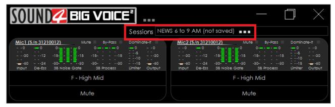
Sessions are used to load configurations for entire shows, and will select presets on the two microphone channels simultaneously. To change the session, click with the mouse cursor on the Sessions filed with the currently used one. This will open a list with all available options, and allow you to select a new one. A click on the name of the session will load it automatically to the device.
