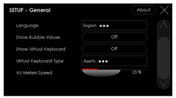
**VU Meter Speed** – This value controls the speed of the onscreen metering and is set in percent. Higher numbers will result in faster metering, though the default of 25% is sufficient.
