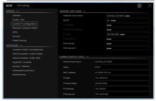
**Network Host Name** – Allows the user to apply the needed changes to the IP configuration - to specify Network host name (that will identify the device on the network), to turn [On] and [Off] the **DHCP** and specify **DNS Server**.
