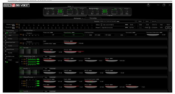
Overview of the two channels (Mic 1 and Mic 2) including channel name, level, mute/de-esser/gate status, currently loaded preset name and etc.
