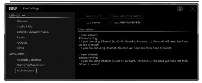
Intended to reset various components if the system. Information as regards the available options can be found in the right part of the screen. Upon selecting any of the reset options, a warning message will appear. To continue with the process, press OK.
