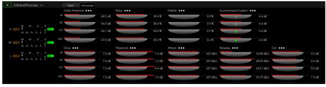
The advanced controls are virtually identical with the basic controls. They add additional metering and access to each band's controls. It includes individual adjustments for each band, as well as an "All" adjustment option that will modify all values at once.
