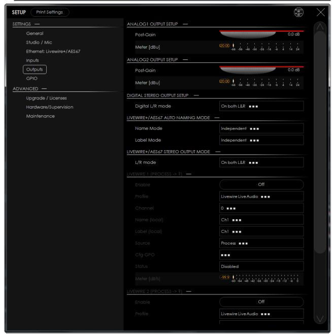
**Analog1 Output Setup/ Analog2 Output Setup** – Allows you to setup the Post Gain, and the meter will indicate the current value.
