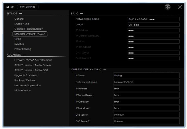
**Basic** – allows the user to specify **Network host name** and to turn [On] and [Off] the **DHCP**. If DHCP is turned Off make sure to specify IP Address, IP Default Gateway, IP Mask, IP broadcast and **DNS Server**.
