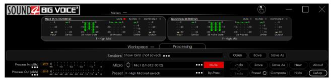
Double click on the desired preset will load it automatically to the device.
