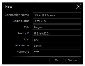
3. If you are not aware of SOUND4 BIG VOICE<sup>2</sup> - Base IP address, it can be seen via the front panel. When the Main screen is on, press the soft button labeled [INFO]. Then using the [Up] and [Down] buttons navigate to IP (2/4) where the IP address of the device will be depicted.
