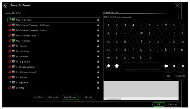
Specify the Preset Name in the relevant line, and press [OK]. Note that when specifying the name, you can either use the interactive keyboard, or write in the field directly.
