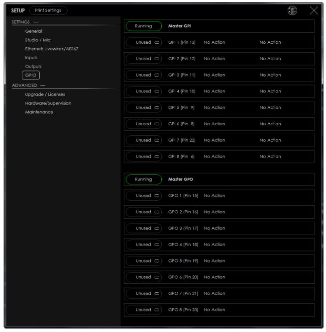
The general purpose inputs and outputs settings are applied through this page. Each GPI/GPO is set individually so as to fit the user's requirements.
