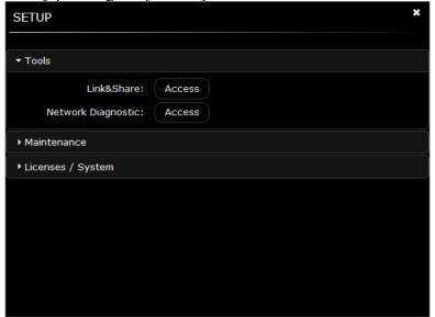
**Link&Share** allows remote control via TCP of BIG VOICE's parameters from an external automation system. This is how the control window looks like:
