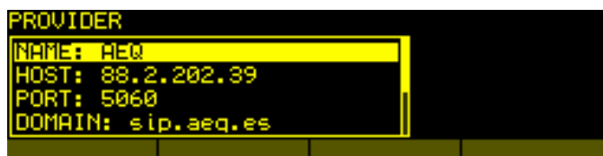
SIP PROVIDERS configuration menu options
