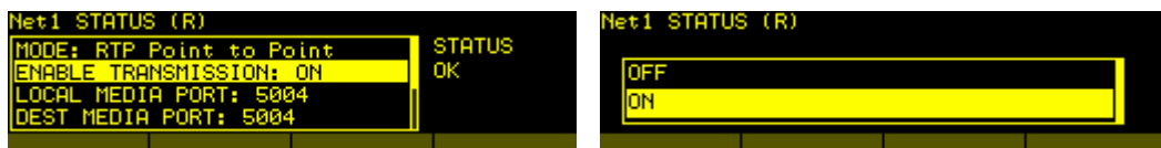
ENABLE TRANSMISSION menu detail
