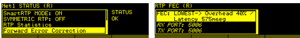
Forward Error Correction menu detail.
