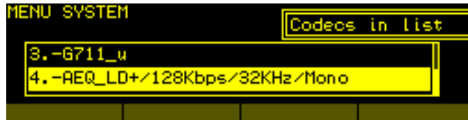
List of algorithms of a SIP CODEC PROFILE and editing options
