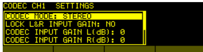
AUDIO CODEC CHANNEL 1 SETTINGS menu detail
