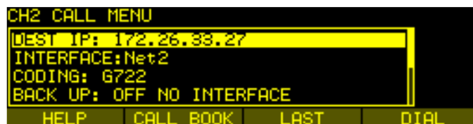
CALL menu detail (IP-RTP mode)
