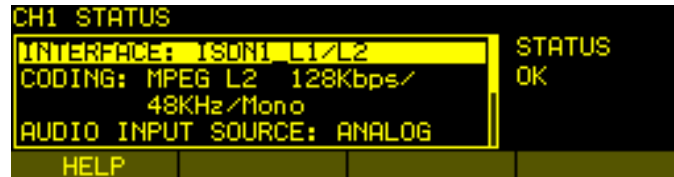
CHANNEL 1 configuration detail
