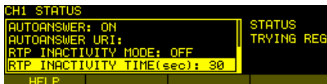
Exclusive configuration options for an IP interface
